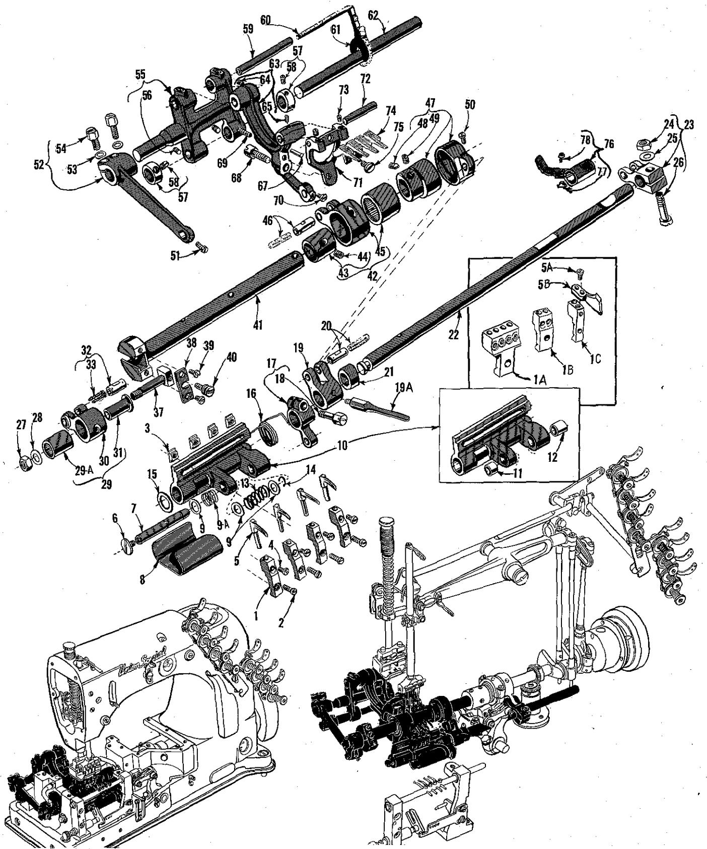
MAIN SHAFT, FEED DRIVING AND LOOPER DRIVING PARTS
