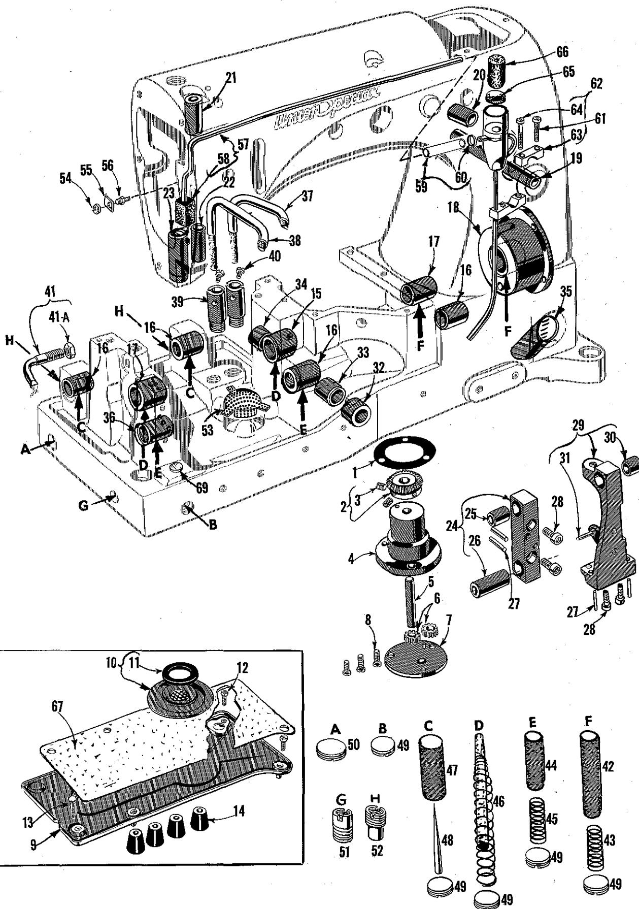
MAIN FRAME, BUSHINGS AND MISCELLANEOUS OILING PARTS
