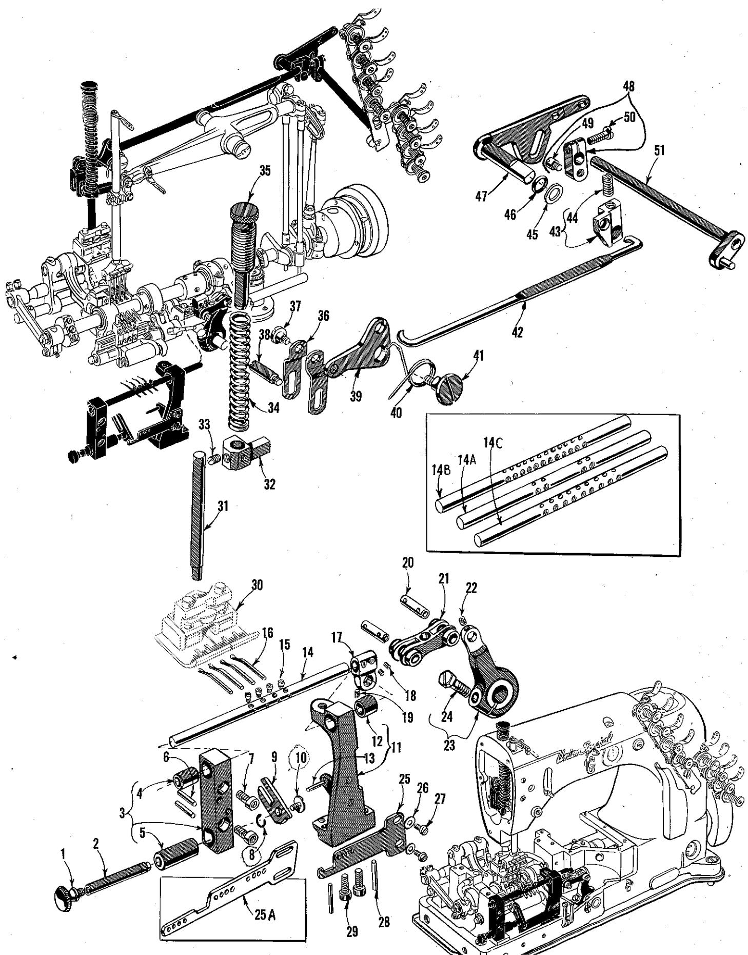
FOOT LIFTER AND RETAINER DRIVING PARTS
